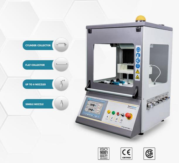
The NE300 Electrospinning Machine, is a compact, flexible lab-scale Electrospinning system. Very similar to the NS 24 but with less emitters (8 nozzles), also has the capacity of single-nozzle production.
